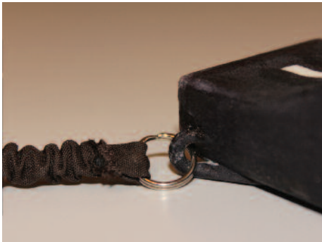
Figure 2. Attachment of the X-shaped elastic teflon harness (below) with a split ring to plastic loops on the side of the logger (above). © Ruben Fijn.
