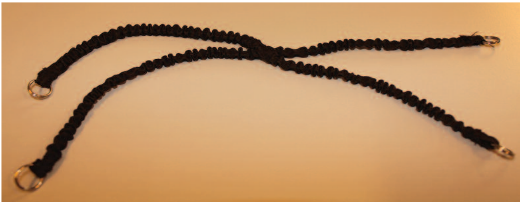
Figure 2. Attachment of the X-shaped elastic teflon harness (below) with a split ring to plastic loops on the side of the logger (above). © Ruben Fijn.
